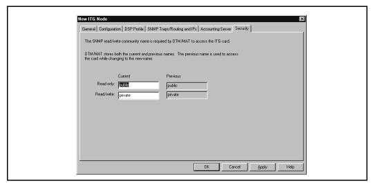
2 Change the default Read only and Read/Write default community names. MAT uses the previous read/write community name to transmit the card properties. The first time you transmit data after changing the password, MAT uses the Previous read/write password. MAT uses the changed password for all following data transmissions.
